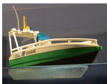
Prototypic flock surface. The silvery shine at the ship hull indicates a kept air layer.
